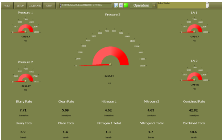
Screen shot of Coiled Tubing DAS Operator Interface
